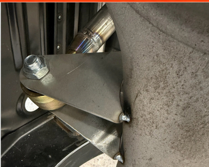
Figure 13 – Tacked axle tabs.
