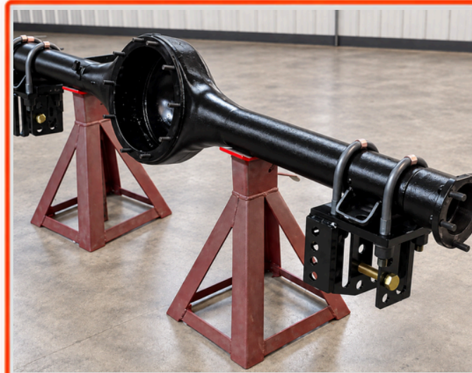
Figure 3 – Both axle brackets installed.
