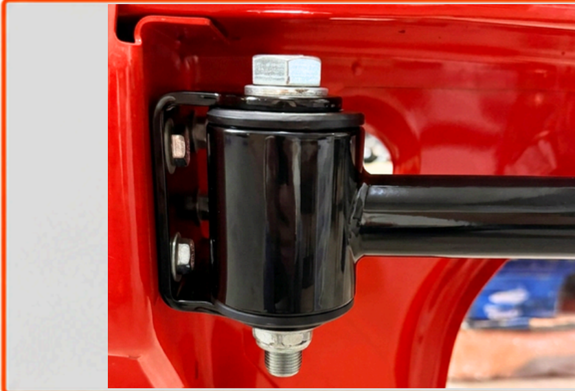
Figure 7 – Forward link bracket installation.
